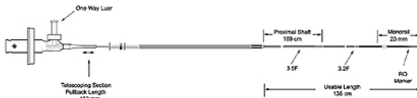
Figure 1: Schematic of Revolution™ 45 MHz IVUS Imaging Catheter
